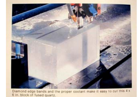
Diamond edge bands and the proper coolant make it easy to cut this 4 x 6 in. block of fused quartz.
